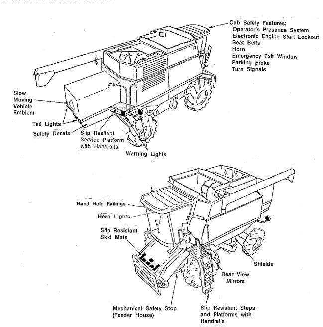
In addition to the safety features shown here, other components and systems, safety signs on the machine, and safety messages and instructions in the operator's manual contribute to the safe operation of this combine when combined with the care and concern of a capable operator.
