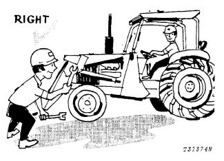
If it is necessary to make checks with the engine running, **ALWAYS USE TWO** service technicians one, the operator, at the controls, the other checking within sight of the operator.
