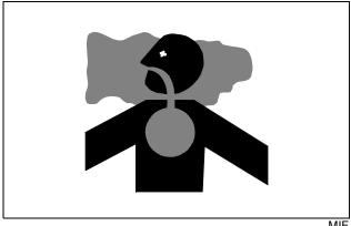
Engine exhaust fumes can cause sickness or death. If it is necessary to run an engine in an enclosed area, remove the exhaust fumes from the area with an exhaust pipe extension.
