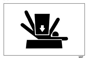
If you must work on a lifted machine or attachment, securely support the machine or attachment.
